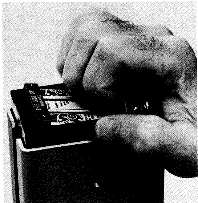
Figure 2-1. Removal of the battery pack.
