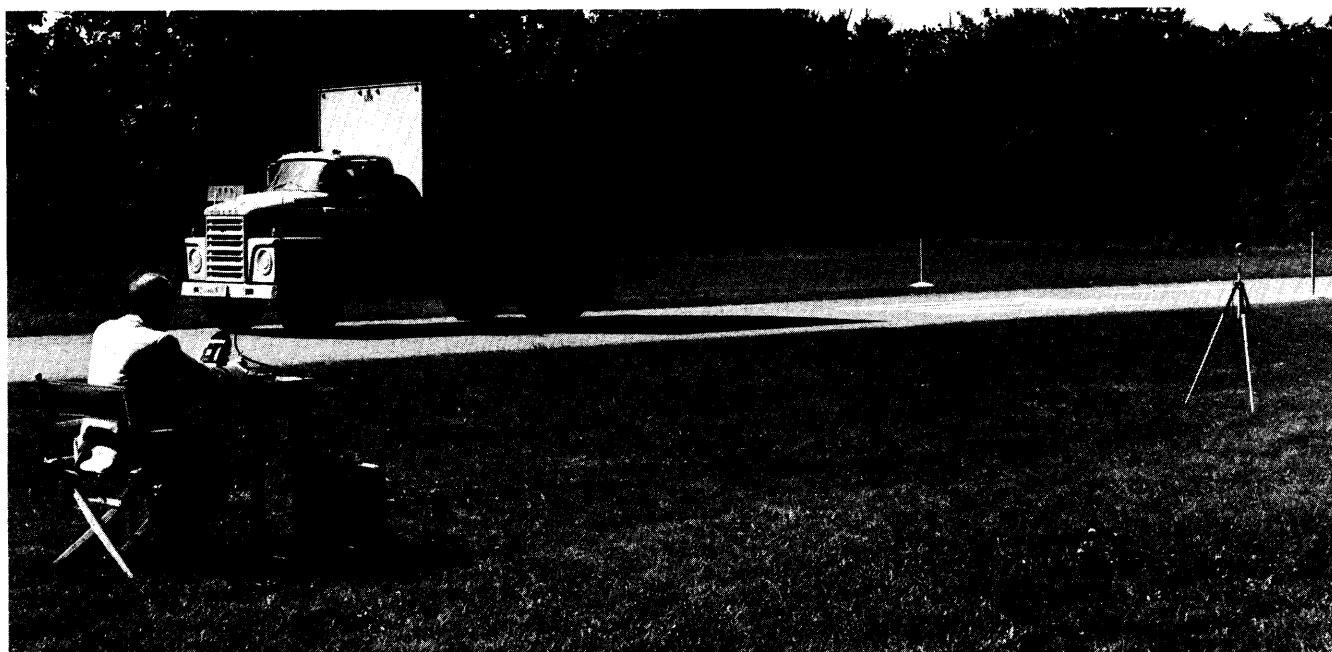
Figure 2-12. Remote location of microphone on tripod is demonstrated by this motor-vehicle noise measurement setup.
